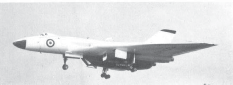
Above: The ill-fated T.S.R.2 Olympus-Vulcan test-bed XA894. Below: The Olympus 593-Vulcan test-bed landing at Filton after its first test-flight. (Top photo: Bristol Siddeley Engines)
