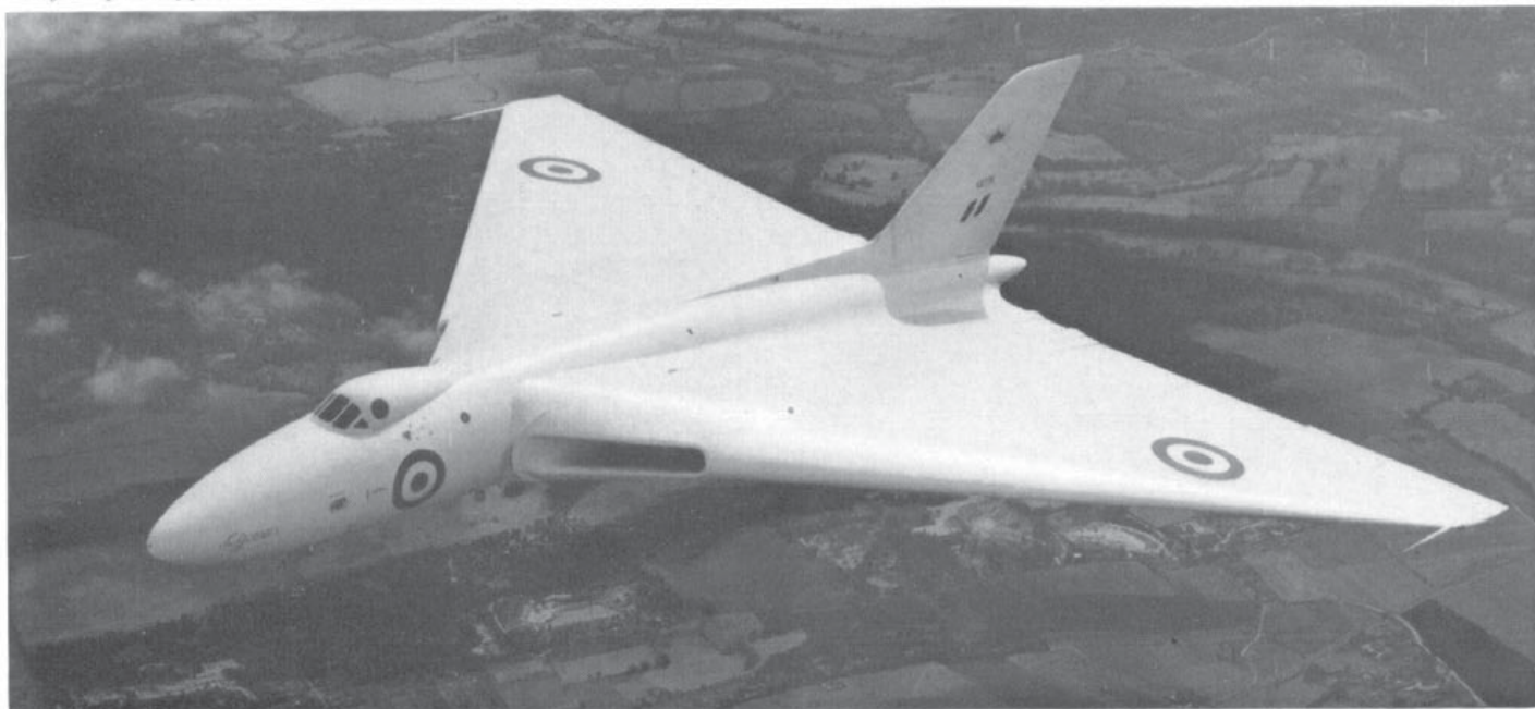
The first prototype Avro 698 Vulcan, VX770, showing the initial, undistorted delta wing planform.
